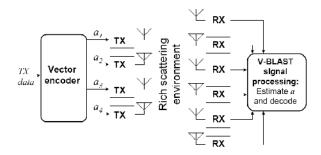
Fig. 1. V-BLAST system block diagram.
